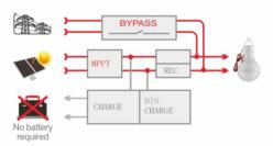
It combines a wide PV input range MPPT controller, can convert solar energy from PV to loads directly and the remaining solar energy converted to batteries synchronously.
